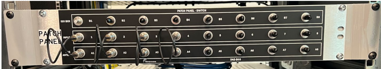
RF Switching Panel
